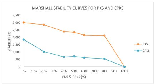
Figure 6: Marshall Stability curve for Crushed Palm kernel Shell and Palm Kernel Shell
