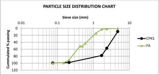
Figure 4: Particle Distribution Curves for Crushed Palm Kernel Shell and Fine Aggregate.
