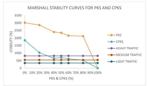
Figure 7: Marshall Stability curve for Crushed Palm kernel Shell and Palm Kernel Shell with specified value for Heavy, Medium and Light Traffic.
