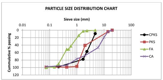
Figure 3: Particle Distribution Curves for Crushed Palm Kernel Shell, Palm Kernel Shell, Fine Aggregate and Coarse Aggregate.
