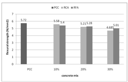
Figure 3: Effect of recycled aggregate on flexural strength of concrete
