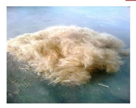
Figure 2: Fiber cut to 30-40 mm sizes
