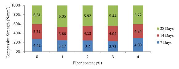
Figure 7: Variation of fiber content with Compressive strength of masonry blocks reinforced with PPF.
