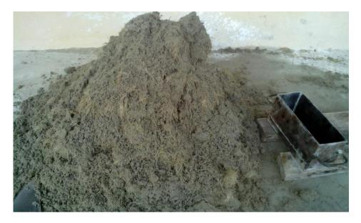
Figure 3: Homogenous mixture of binders, sand, water and fiber ready for casting.
