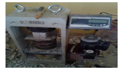
Figure 5: Compressive strength testing of block specimens
