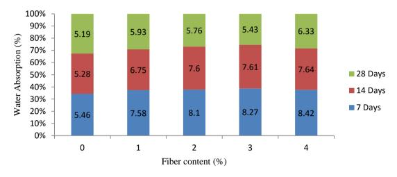
Figure 10: Variation of fiber content with water absorption of masonry blocks reinforced with PPF
