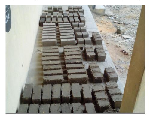
Figure 4: Wet block specimens after casting
