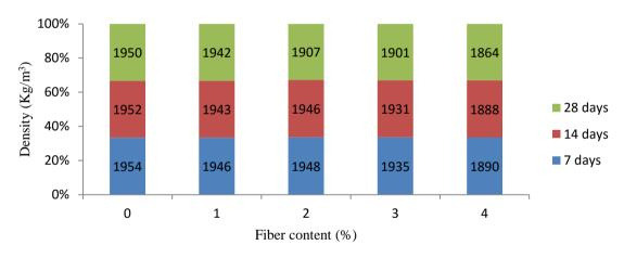
Figure 9: Variation of fiber content with density of masonry blocks reinforced with PPF
