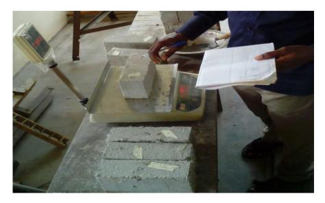
Figure 6: Weighing of Block Samples for Density Determination
