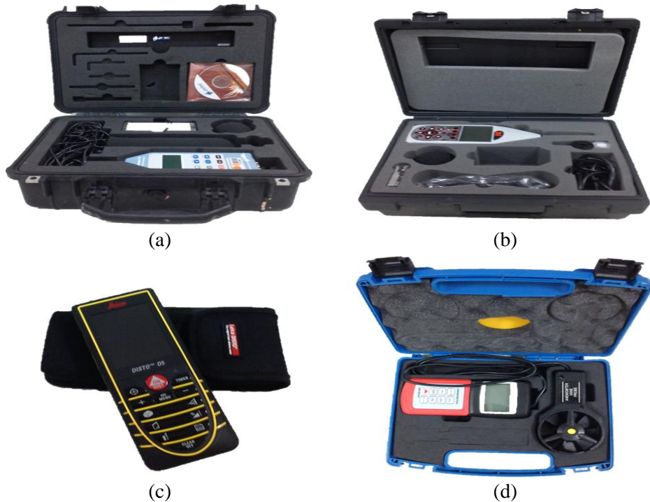
Figure 3: Required instrumentations (a) Sound level meter - Type 1, (b) Sound level meter - Type 2, (c) Distometer and (d) Anemometer
