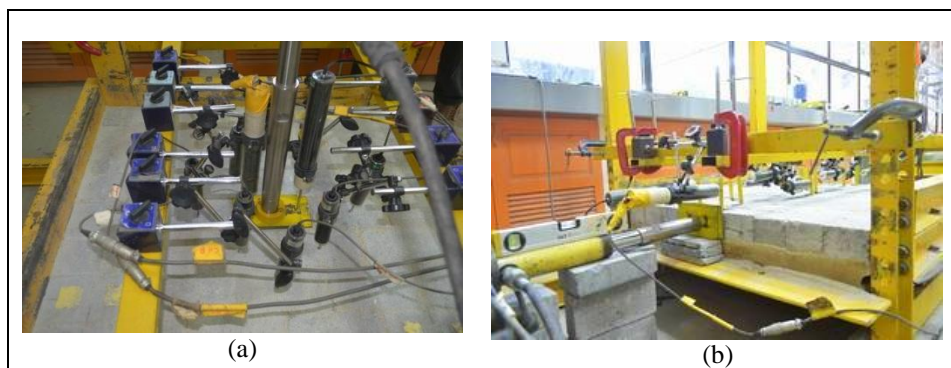
Figure 3: (a) Push-in loading test and (b) Horizontal loading test
