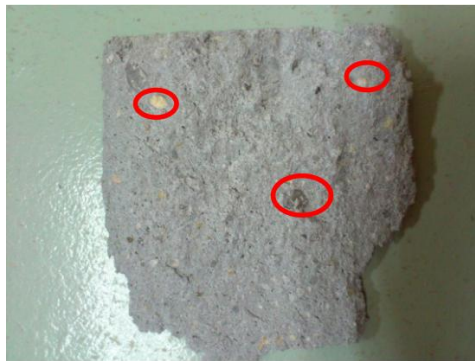
Figure 7: Coarser sand inside the lightweight foamed concrete specimens
