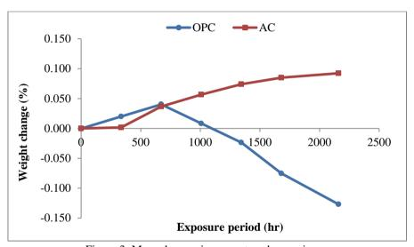
Figure 3: Mass changes in concrete cube specimens
