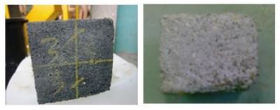
Figure 2: Appearance of specimens after immersed in 5% sulphuric acid solution
