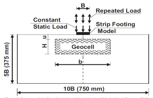
Figure 3: Geometry of the Geocell-reinforced foundation bed (Moghaddas & Dawson, 2012).
