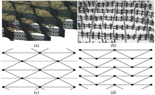
Figure 2: The typical configurations of geocell reinforcement elements. (a) Perforated geocell (Bathurst and Jarrett, 1998). (b) Handmade geocell (Dash *et al.*, 2003). (c) Handmade geocell diamond pattern (Dash *et al.*, 2003). (d) Handmade geocell chevron pattern (Dash *et al.*, 2003).
