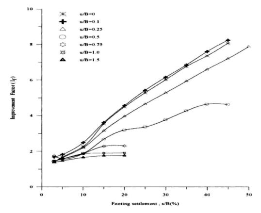
Figure 5: Variation of improvement factors with settlement for different depths of placement of geocell (Dash et.al, 2001).
