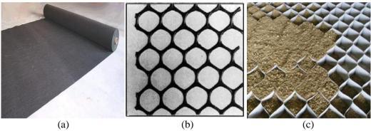
Figure 1: Various kinds of geosynthetics (a) Geotextile (Pokharel, 2010), (b) Geogrid (Alamshahi and Hataf, 2009), (c) Geocell (Yang *et al.*, 2012).
