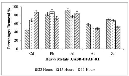
Figure 6: Removal percantages of heavy metals on combined UASB-DFAF(R1) reactors at different HRT
