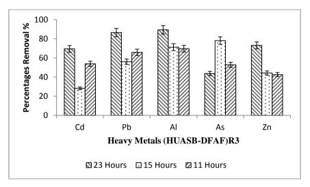
Figure 8: Removal percantages of heavy metals on combined HUASB-DFAF(R3) reactor at different HRT
