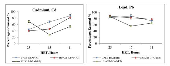
Figure 9: Comparison removal percentages of Cadmium between combined system and HRT.
