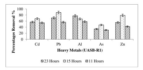
Figure 3: Removal percantages of heavy metals in UASB-R1 reactors at different HRT
