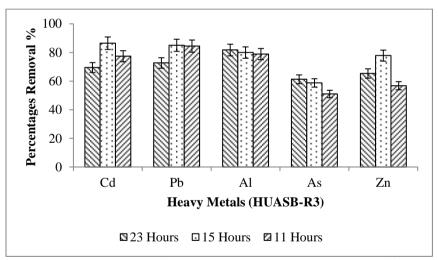
Figure 5: Removal percantages of heavy metals in HUASB-R3 reactors at different HRT
