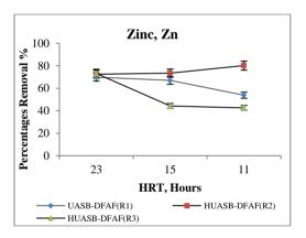
Figure 13: Comparison removal percentages of Zinc between combined system and HRT.
