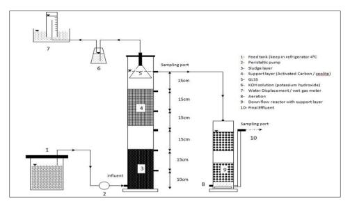
Figure.1: Schematic diagram of UASB-DFAF and HUASB-DFAF reactor
