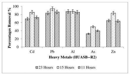
Figure 4: Removal percentages of heavy metals in HUASB-R2 reactors at different HRT
