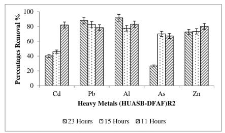
Figure 7: Removal percantages of heavy metals on combined HUASB-DFAF(R2) reactor at different HRT
