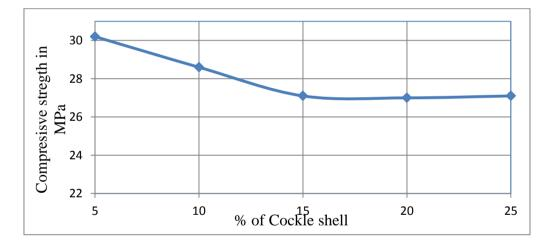
Figure 10 (a): Compressive strength of concrete with different percentage of cockle shell (granite powder 25% fixed)
