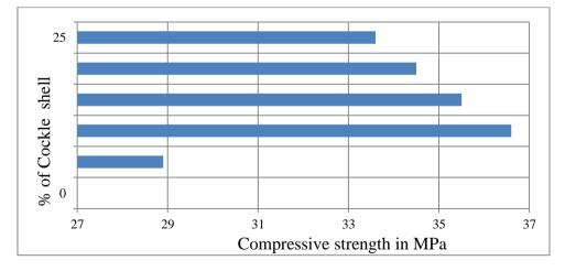
Figure 7 (b): Compressive strength of concrete with varying percentage of cockle shell (granite powder 10% fixed)
