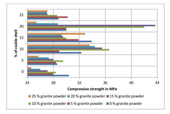
Figure 11 (b): Compressive strengths of concrete with fixed granite powder replacement
