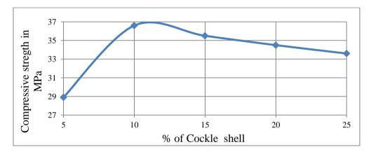
Figure 7 (a): Compressive strength of concrete with varying percentage of cockle shell (granite powder 10% fixed)
