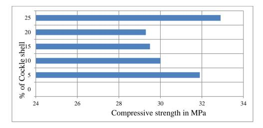
Figure 8 (b): Compressive strength of concrete with different percentage of cockle shell (granite powder 15% fixed)
