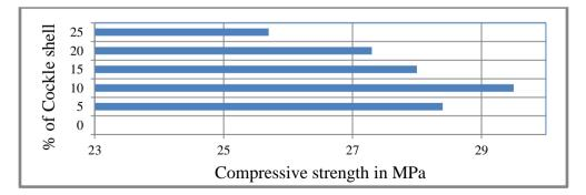
Figure 6 (b): Compressive strength of concrete with different percentages of cockle shell (granite powder 5% fixed)
