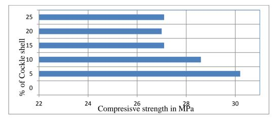
Figure 10 (b): Compressive strength of concrete at different percentage of cockle shell (granite powder 25% fixed)
