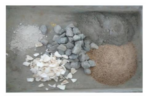
Figure 3: Ingredients of concrete including cockle shell and granite powder
