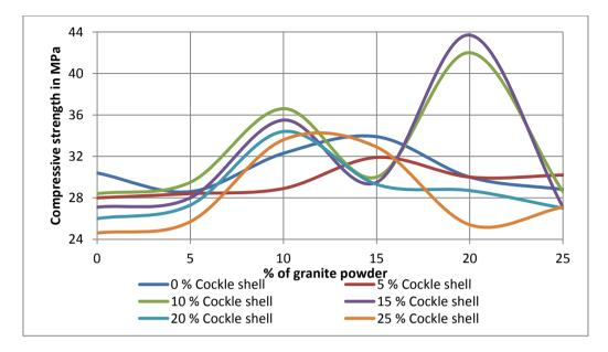
Figure 11 (a): Compressive strengths of concrete with fixed granite powder replacement
