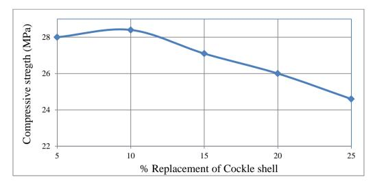
Figure 5 (a): Compressive strength of concrete at different percentage of cockle shell
