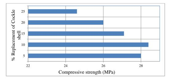
Figure 5 (b): Compressive strength of concrete at different percentage of cockle shell
