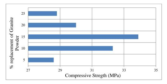
Figure 4 (b): Compressive strength of concrete at different percentage of granite powder
