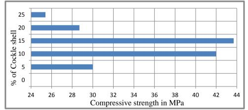
Figure 9 (b): Compressive strength of concrete with different percentage of cockle shell (granite powder 20% fixed)
