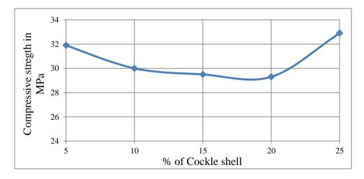
Figure 8 (a): Compressive Strength of concrete with different percentage of cockle shell (granite powder 15% fixed)
