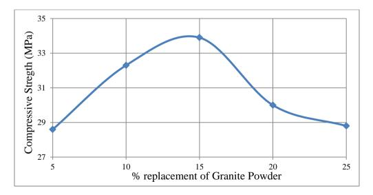
Figure 4 (a): Compressive strength of concrete at different percentage of granite powder
