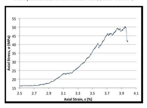
Figure 3: Non-linear Deformation of Kuala Lumpur Limestone
