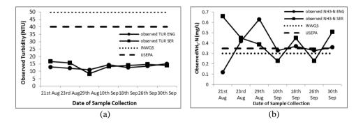
Figure 3: Observed data of a) Turbidity and b) NH<sub>3</sub>-N compared to standards for Engineering and Serumpun Lake
