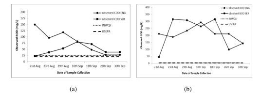
Figure 2: Observed data of a) BOD and b) COD for Engineering and Serumpun Lakes compared to INWQS and USEPA standards.
