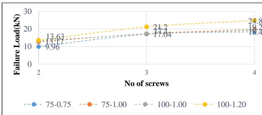
Figure 9: Failure load vs number of screw arranged not parallel with the load
