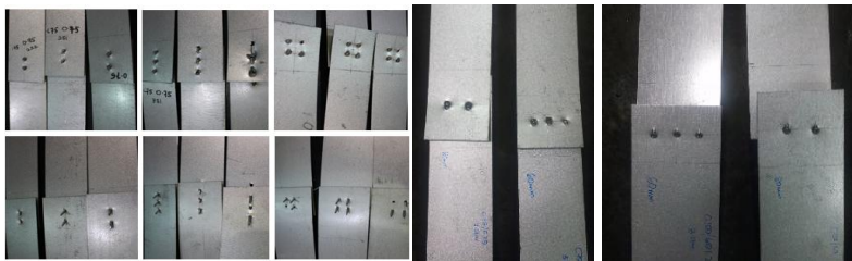
Figure 10: Failure mode of screw connections
