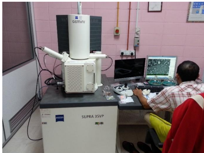
Figure 5: Field emission scanning electron microscope (FESEM) test
