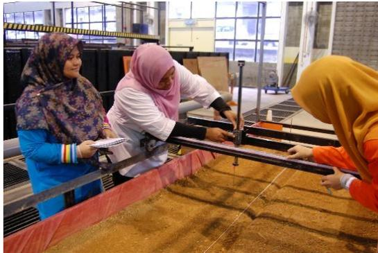
Figure 1: Measurement of river channel profile using digital point gauge
