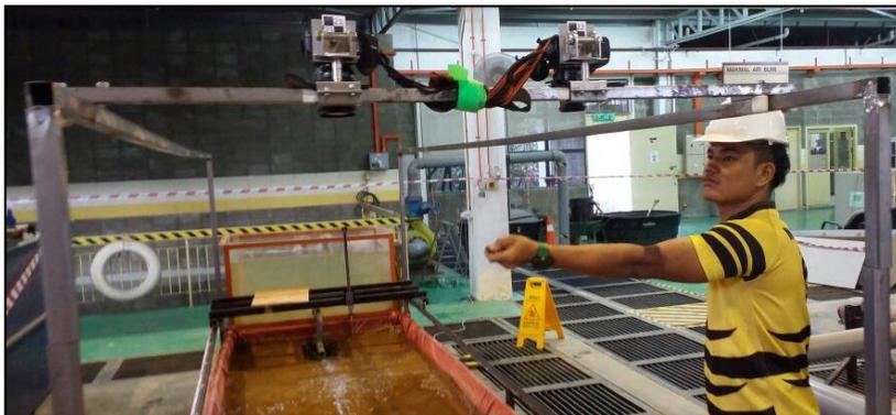
Figure 5: Image Acquisition Setup Using DRCP Technique
