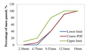
Figure 4: Sieve analysis of coarse POC aggregates
