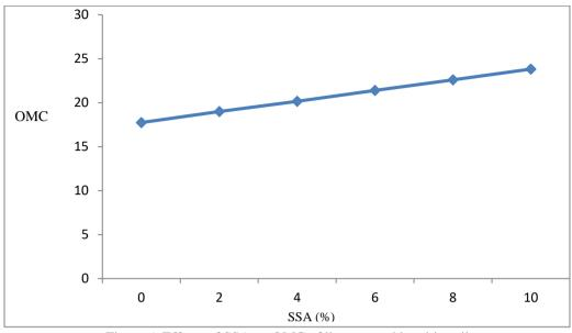
Figure 6. Effects of SSA on OMC of lime-treated lateritic soil
