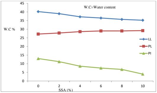
Figure 4. Effects of SSA on atterberg limits of lime-treated lateritic soil
