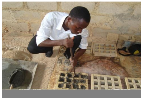
Figure 5: Compacting the Mortar
