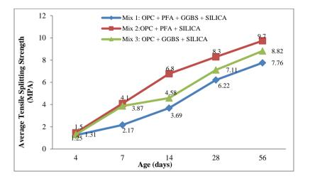
Figure 5: Average of tensile splitting strength of different concrete mix and age for 100% QD
