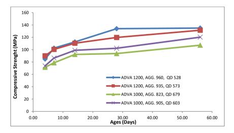
Figure 6: Variation of compressive strength with curing times for different ADVA, AGG. & QD contents at 155 H2O & 436 OPC m3/kg at PFA (30 %) +SILICA (6 %)
