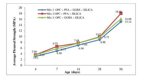
Figure 4: Average of flexural strength of different concrete mix and age for 100% QD
