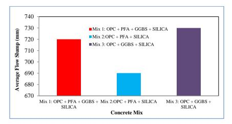
Figure 1: Variation of slump value of fresh concrete with different concrete mixes for 100% QD
