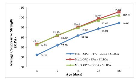
Figure 3: Average of compressive strength of different concrete mix and age for 100% QD
