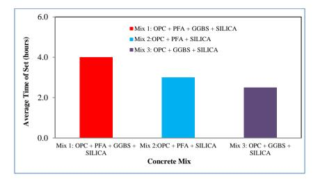
Figure 2: Effect of different constituents concrete mixes in initial time of set for 100% QD
