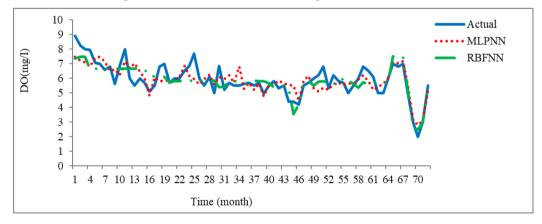
Figure 6: Actual and modelled DO (mg/l) in water at turbine discharge
