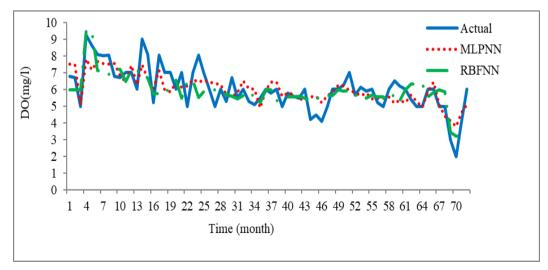
Figure 3: Actual and modelled DO (mg/l) in water at power intake
