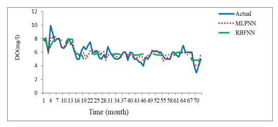
Figure 4: Actual and modelled DO (mg/l) in water at boatyard
