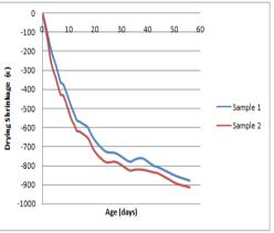
Figure 14: Drying shrinkage of M<sub>3</sub> over age
