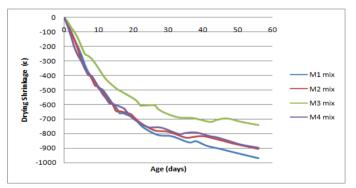
Figure 16: Drying shrinkage of concrete over age
