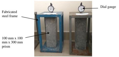
Figure 5: Drying shrinkage measurement
