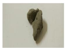
Figure 1: Coated foamed aggregates
