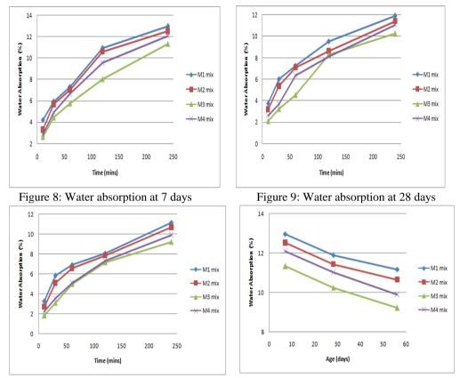
Figure 10: Water absorption at 56 days Figure 11: Water absorption of concrete over Age
