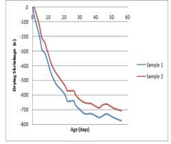
Figure 13: Drying shrinkage of  $M_2$  over age
