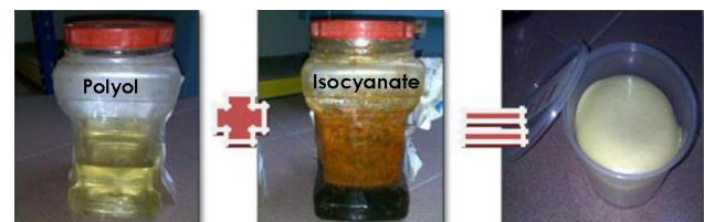
Figure 4 Combination of polyol and isocyanate to form polyurethane foam
