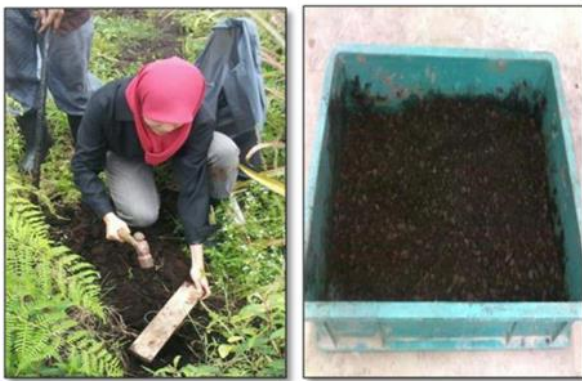
Figure 2 Peat soil sample; (a) undisturbed sample of peat soil taken at site, (b) The disturbed sample of peat soil
