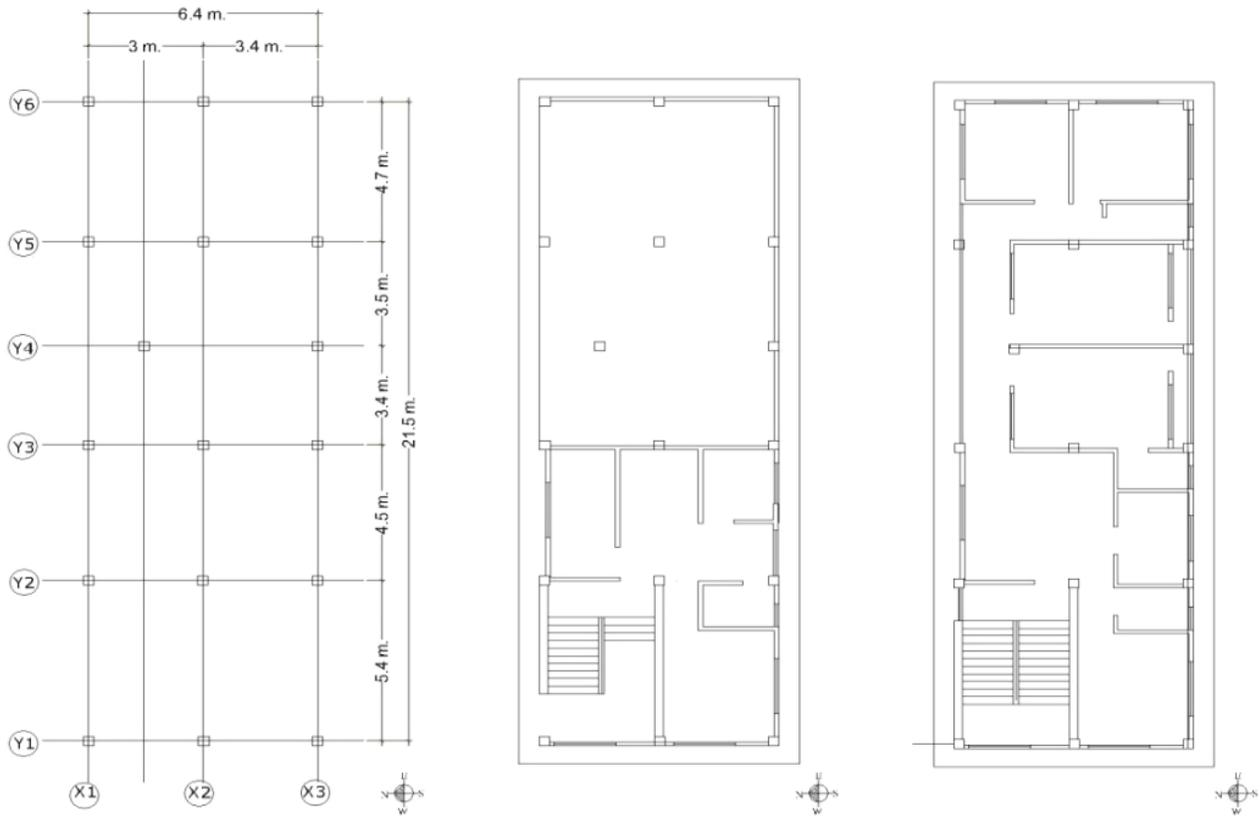
Figure 4 Column layout, GF and Typical Floor plan of the building
