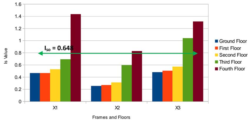
Figure- 8:  $I_s$  and  $I_{so}$  Index comparison at longitudinal (X) direction
