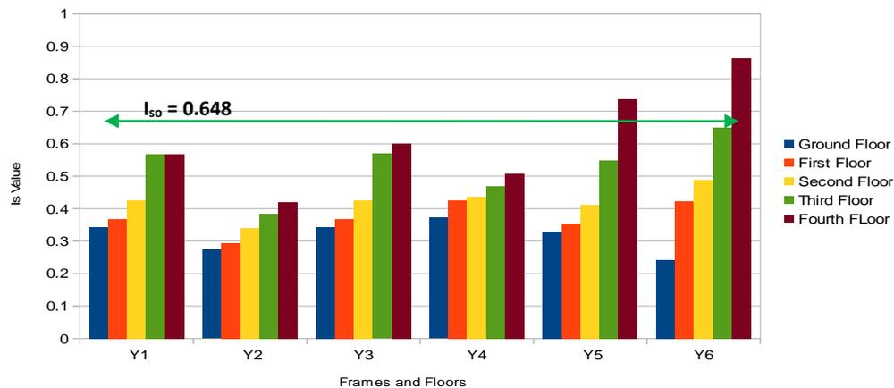
**Figure- 7:**  $I_s$  and  $I_{so}$  index comparison at transverse (Y) direction
