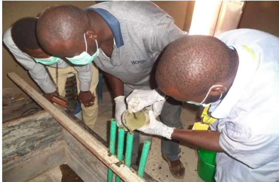
Figure 1 Pouring of the mixed Epoxy mixture into moulds
