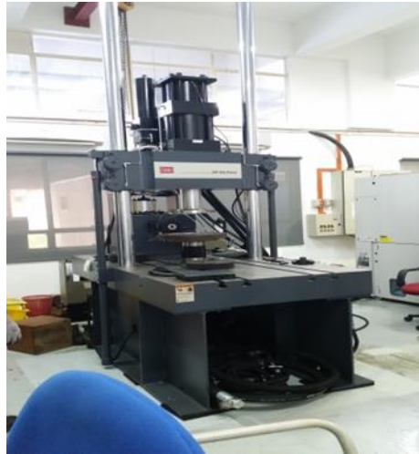
Figure 4 Servo Hydraulic MTS322 testing machine for Compression and Dynamic Load Test
