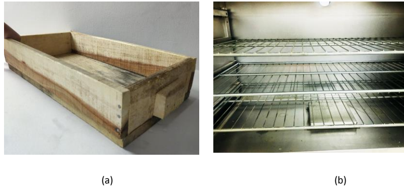
Figure 3 Mold for plastic shrinkage test (500 X 250 X 75) mm; (b) Temperature controlled chamber
