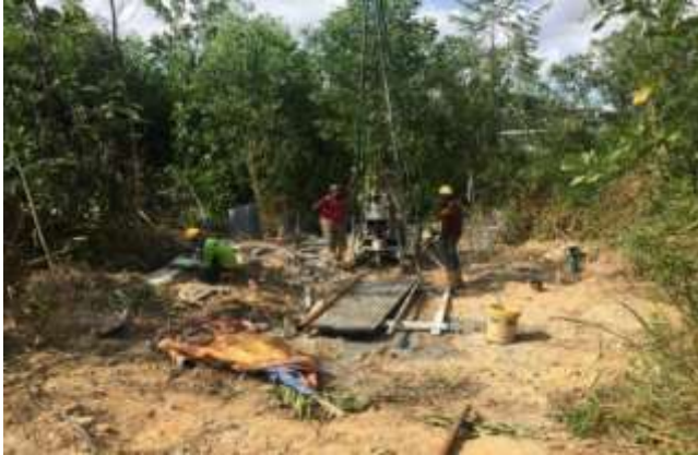
Figure 4 Field exploration by using deep rotary boring machine
