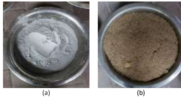
Figure 1: (a) Fly ash (Class F) & (b) Wood powder used for the study
