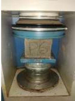
Figure 3: Testing for compressive strength
