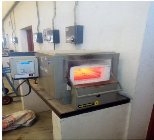
Plate 6: Electric Furnace used for Fire Resistance Test
