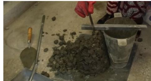
Plate 5: Slump Test at 25% Replacement
