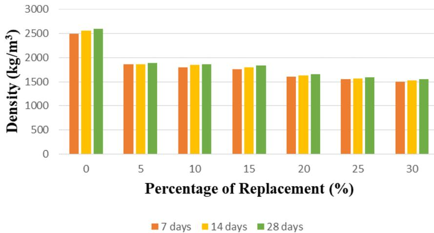
Figure 2. Density of Unfired Concrete Cubes Corresponding to Percentage of Replacement
