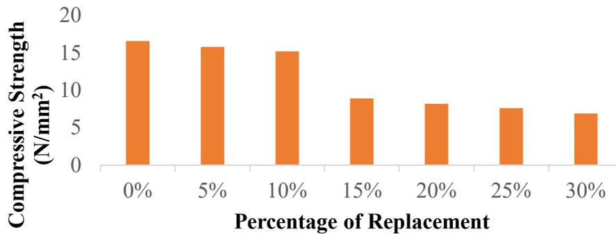
Figure 5: Compressive Strength of Fired Concrete Cubes Corresponding to 28 days Curing Age at Different RPA Percentage Replacement.
