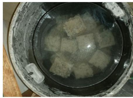
Plate 3: Plate 4: Curing of concrete Cubes
