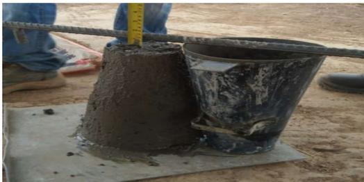
Plate 4: Slump Test at 0% Replacement
