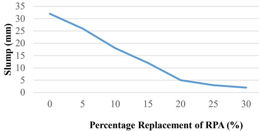
Figure 1: Slump of Fresh Concrete
