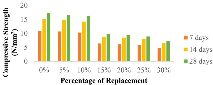
Figure 4: Compressive Strength of Concrete Cubes at Varying Percentage of Replacement
