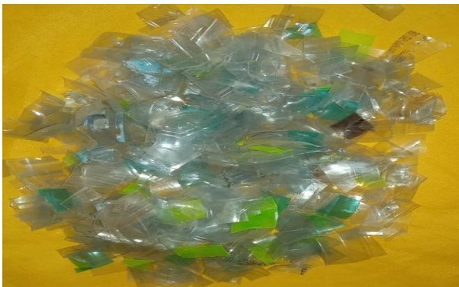
Plate 1: Samples of Waste Plastic Bottles as Coarse Aggregates
