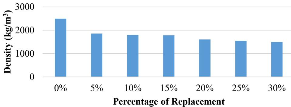
Figure 3: Density of Fired Concrete Cubes Corresponding to Percentage of Replacement
