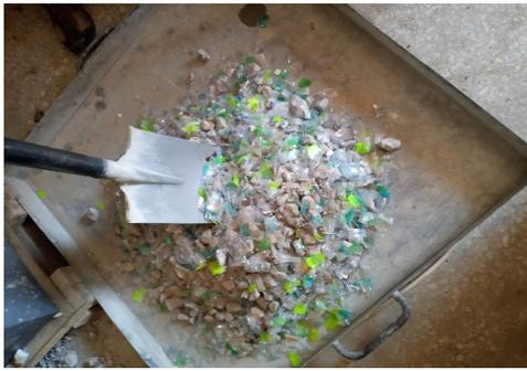
Plate 2: Hand Mixing of Concrete
