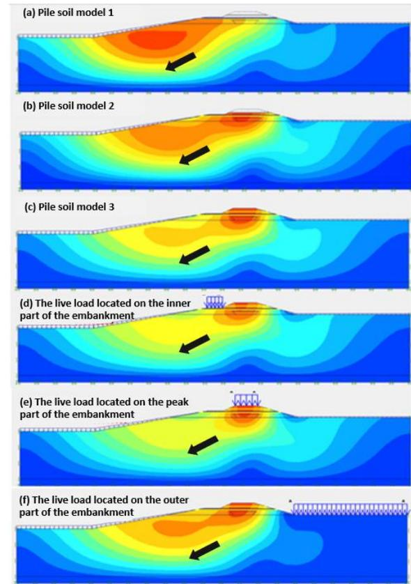
**Figure 5** Total Soil Displacement Contour in Each Construction Stage
