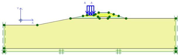
Figure 2 Live Load Placement on the Inner Part of Manyar Pond
