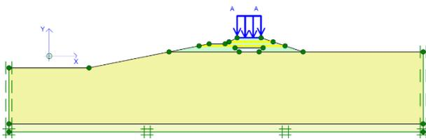
Figure 3 Live Load Placement on the Top Part of Manyar Pond
