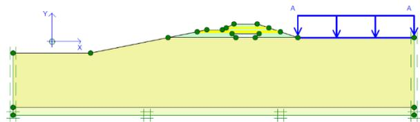
Figure 4 Live Load Placement on the Outer Part of Manyar Pond
