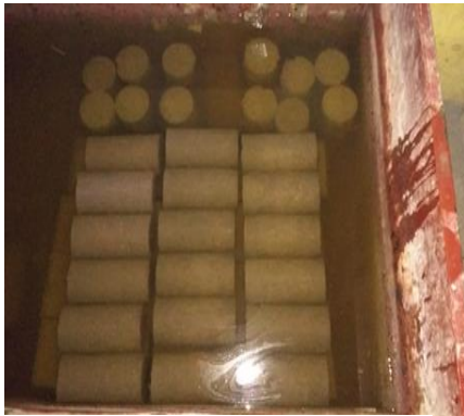
Figure 11. Curing condition. (In lab)
