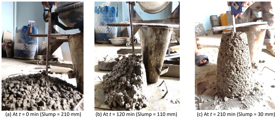
Figure 5 Slump test of concrete without admixture
