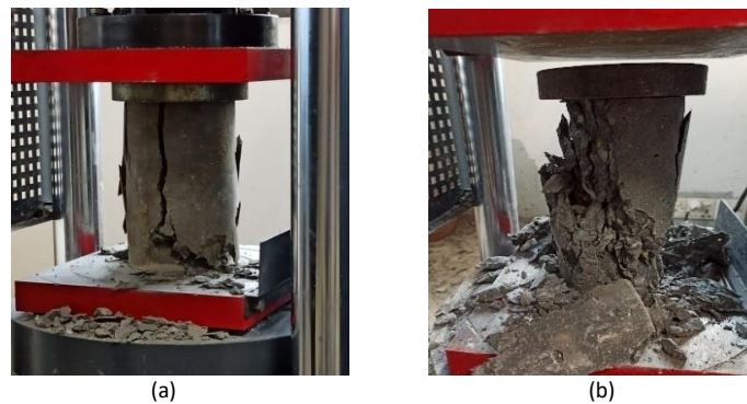
Figure 6 Compressive test (a) specimen under loads and (b) specimen damage after releasing compression load
