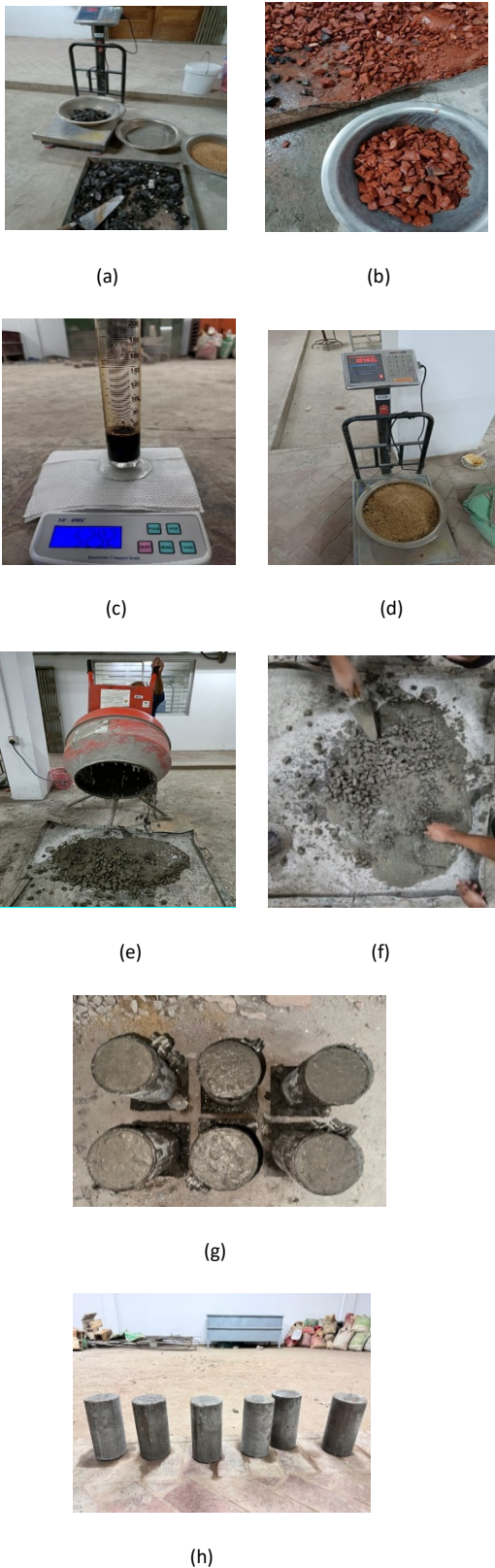
Figure 4 Concrete Casting (a) Slag Weighing (b) Recycled Brick Chips Weighing (c) Superplasticizer (ASTM C-494: Type A & F) measuring as per requirement (d) Sylhet Sand Weighing (e) Concrete Mixing Machine (f) Mixing the fresh concrete after coming out from the mixing machine for homogenous concrete mix (g) Freshly Casted Concrete Cylinder (h) Concrete after 28days curing.
