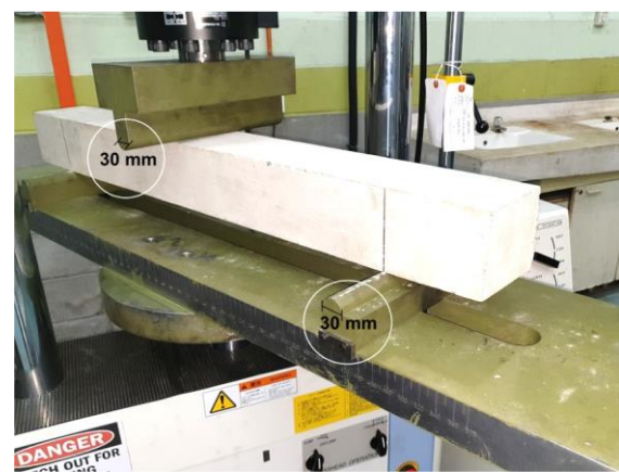
Figure 1 Three-point bending test configuration for fatigue testing.
