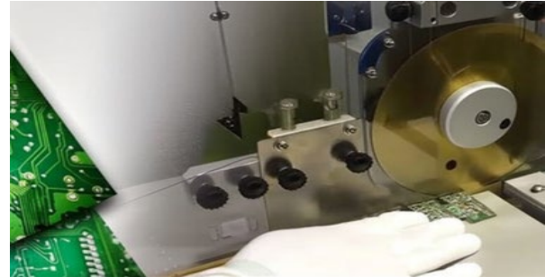
Figure 8 Cutting of PCB
