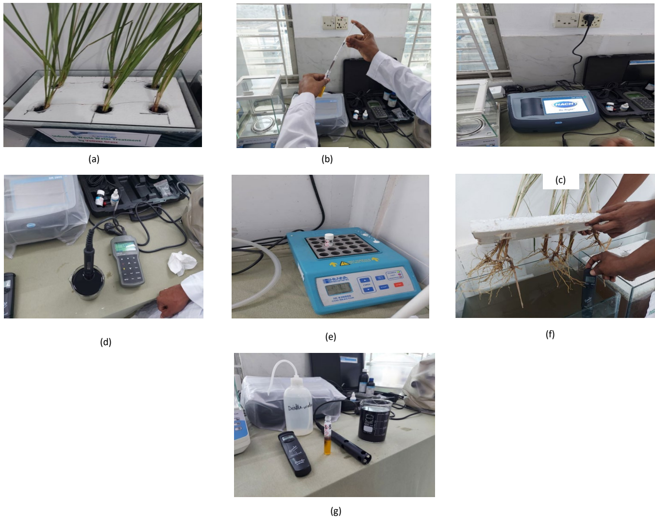
Figure 2 (a) Vetiver plants inside the holes, and Total Dissolved Solids (TDS) test apparatus, (b) Water Sample Preparation, (c) Colorimetric Analysis using Spectrophotometer, (d) Dissolved oxygen (DO) meter, (e) COD Reactor, (f) Vetiver Plant Growth Observation, and (g) pH, Temperature, Electrical Conductivity (EC).
