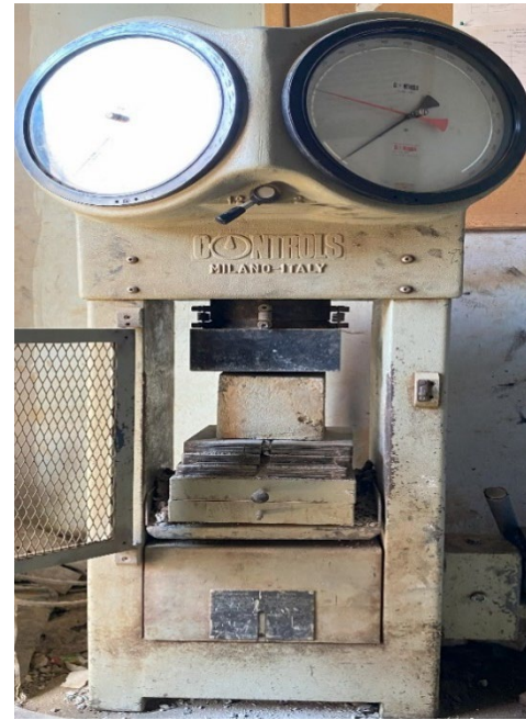
Figure 2 Compression testing machine with cube specimen
