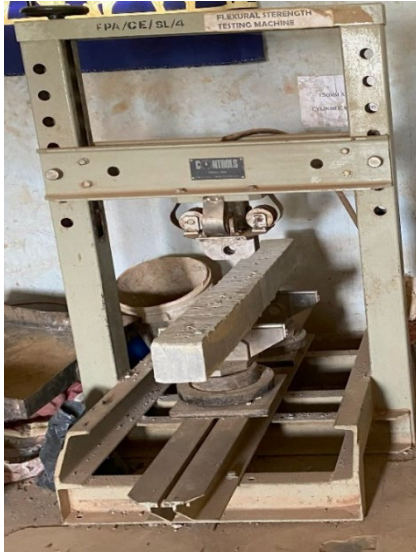
Figure 3 Testing of specimens for modulus of rupture
