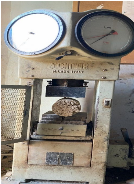
Figure 4 Testing of specimens for splitting tensile strength.
