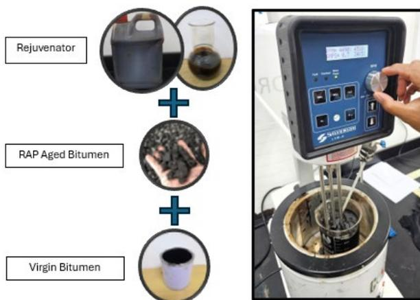
**Figure 2** Mixing of Rejuvenator, Recovered RAP Binder and Virgin Bitumen
