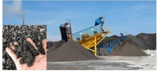
**Figure 1** RAP after Fractioning and Screening into Different Sizes
