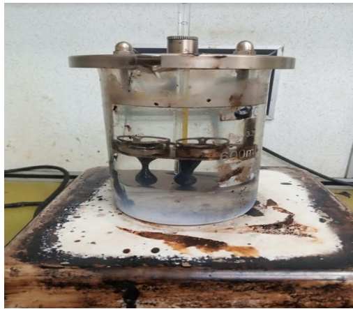
Figure 3 Testing of softening point
