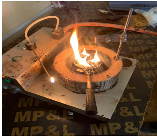
Figure 6 Testing of the fire point
