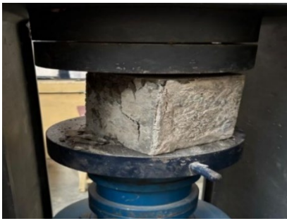
Figure 1 compression testing of cube specimen
