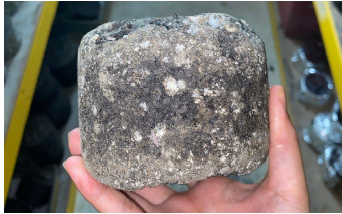
Figure 11 Cantabro sample after testing
